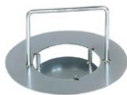
3. Three Prong Cup Puller [No. 200] Zinc plated steel with a red rubber handle; Place, twist and pull to remove the cup. Size: approx. 24" Works only on 250AL cups.
